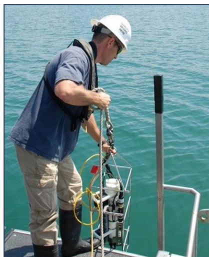
Photograph 4. Water column profile sampling using a CTD profiler.
