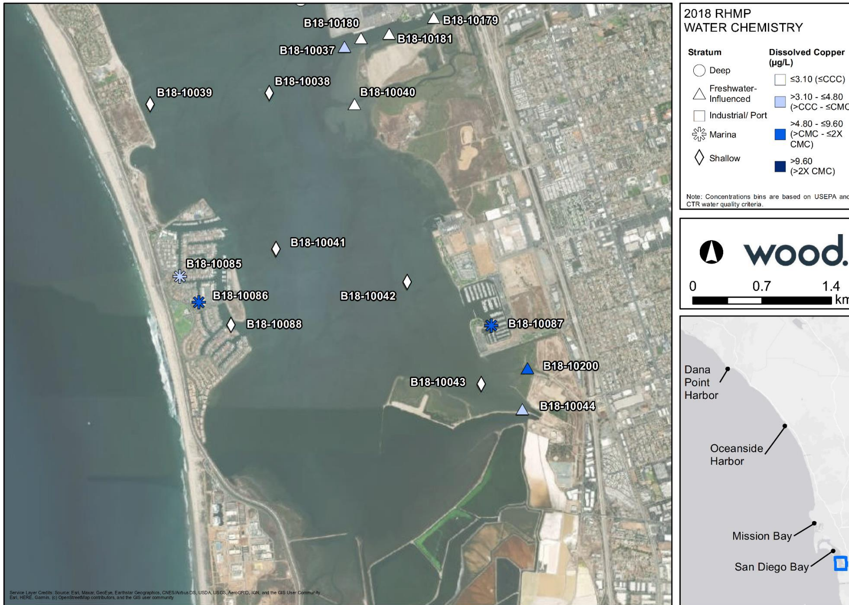
Figure 3-7f. Distribution of Dissolved Copper Concentrations in Surface Waters of South San Diego Bay
