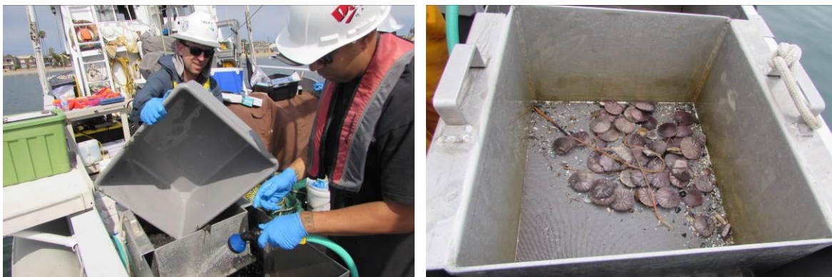
Photographs 7 and 8. Processing a sediment grab through the 1-mm sieve for benthic infauna analyses
