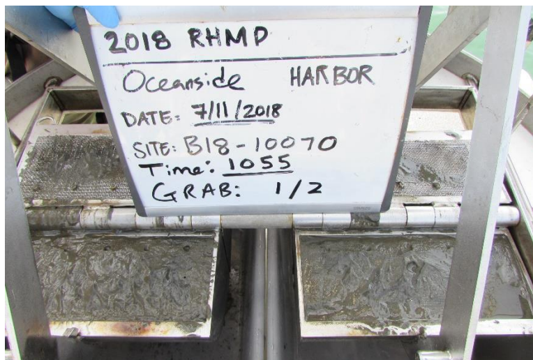
Photograph 6. TVV grab showing an acceptable intact sediment sample for processing
