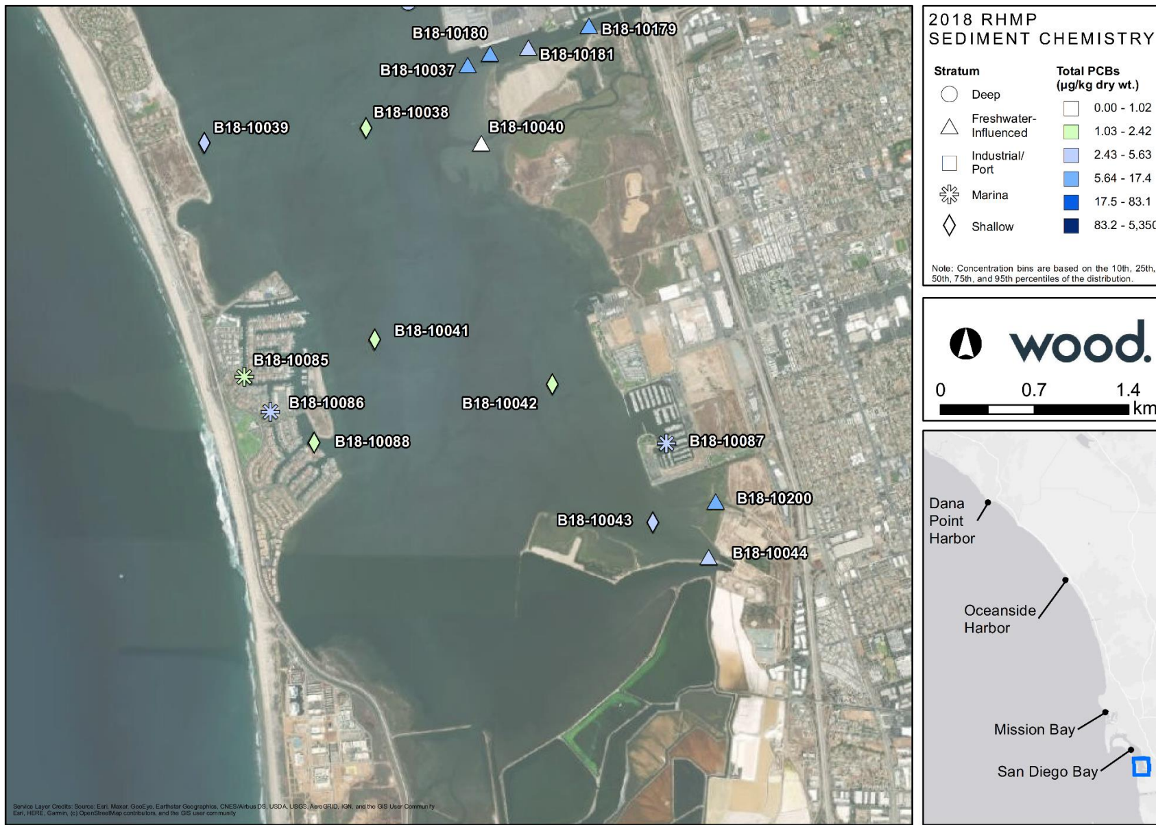
Figure 3-31f. Spatial Distribution of Sediment Total PCB Concentrations in South San Diego Bay
