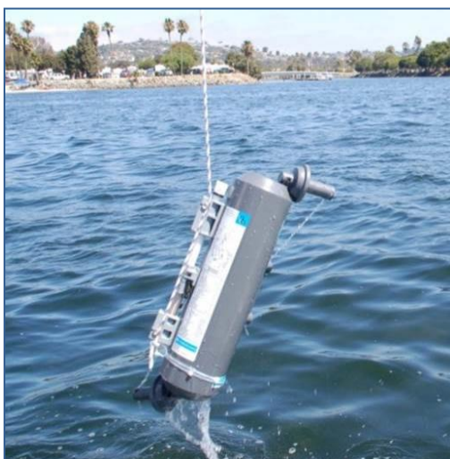
Photographs 1 and 2. Collection of water samples using a Niskin bottle and subsequent processing aboard the R/V Early Bird II
