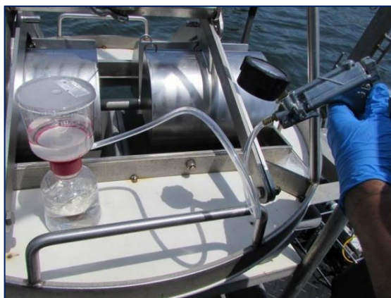
Photograph 3. Field filtration for analysis of dissolved trace metals
