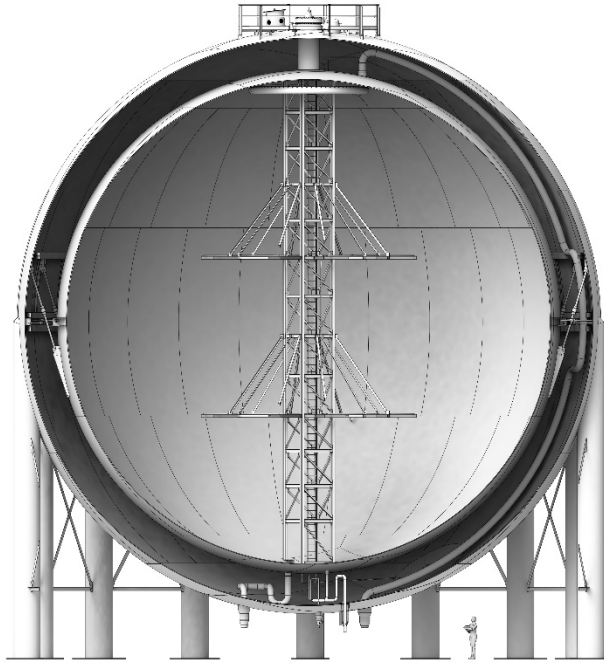
Figure 2. Cutaway of the New NASA Sphere Showing the IRAS Heat Exchanger Support Tower (Courtesy CB&I)
