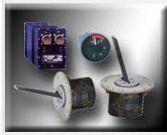
Stall warning vanes electronic processing units & cockpit display
