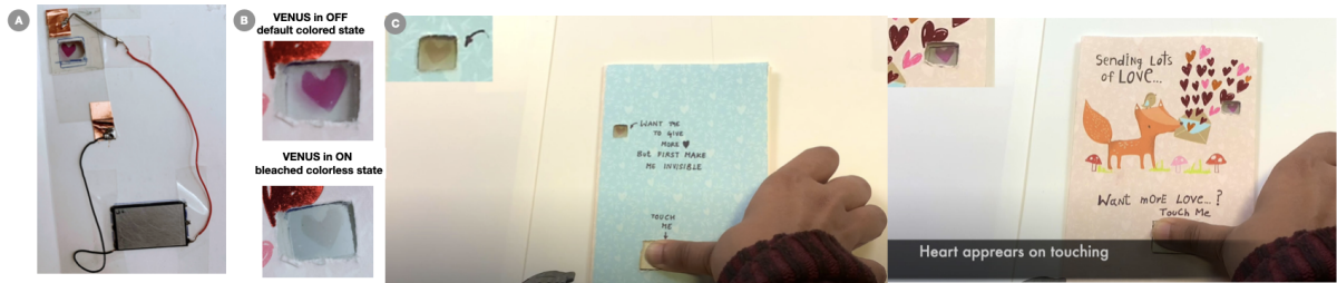
Figure 5.20: Hand touch powered interactive cards a. TEG connected to VENUS display embedded in card b. VENUS display in onset and clear mode c. Interactions that change the state of VENUS display with respect to card
