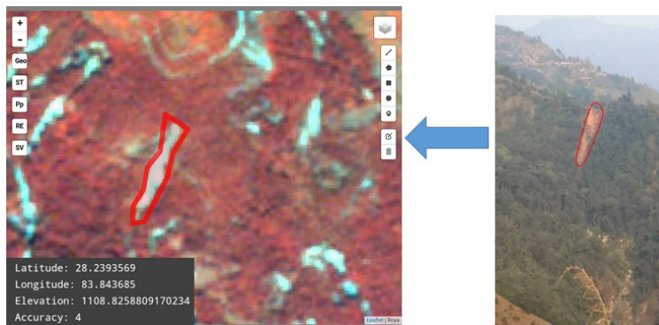
Figure 12. Data collection from a distance where access was difficult but location was easy on the map using geolocation and satellite imagery.
