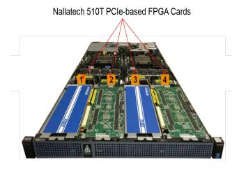
Figure 2.14: Nallatech FPGA-Accelerated Compute Node [13]
