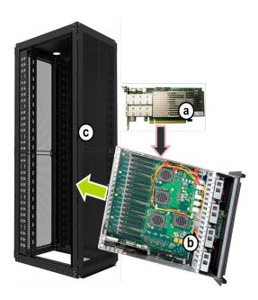
Figure 3.9: Building an FPGA Rack Using off-the-shelf HW: (a) FPGA module with 16 GB DRAM. (b) 2U Rack chassis [22] with 18 FPGA modules. (c) 42U Data Center Rack
