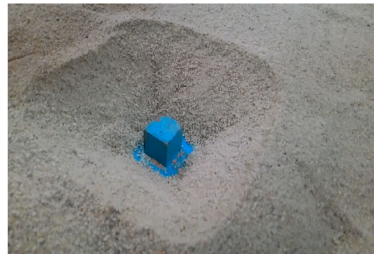
Fig. 10 IBS footing in dense sand after soil failure
