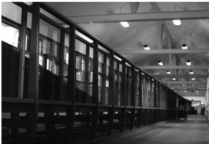
Fig. 2. Wave flume at IBW PAN in Gdańsk – “IBW PAN 2010” experiment (photo by Ł. Sobczak).
