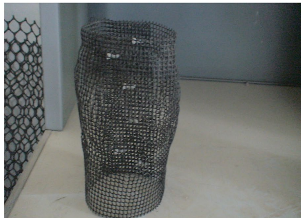
b Geomesh deformation after compression loading test
