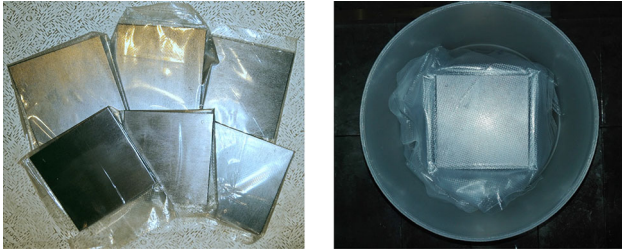
Fig. 3 (Left) the Ta sample consists of six tiles. (Right) the tiles arranged inside the Marinelli
