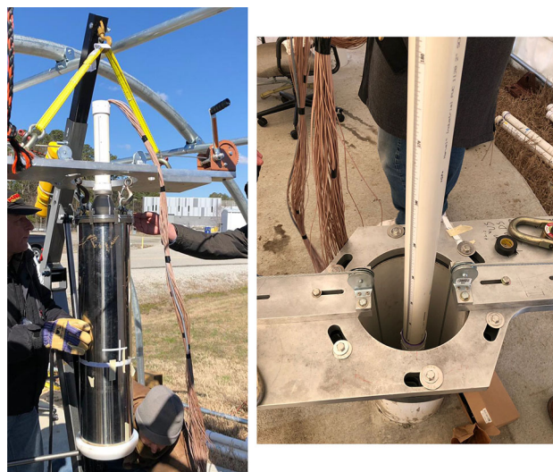
Fig. 2 Some pictures of BDX-Mini detector positioning phases. Left Panel shows the BDX-mini detector inside the stainless-steel watertight cylindrical vessel. Right Panel shows the detector lowering phase in the pipe: a PVC segment with the attached tape is clearly visible
