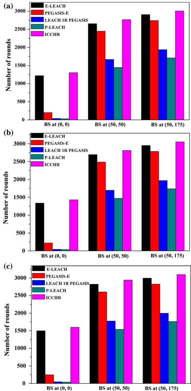
Fig. 6 The comparisons of five algorithms using FND, HND, and AND three metrics for BS locations at (0, 0), (50, 50), and (50, 175)
