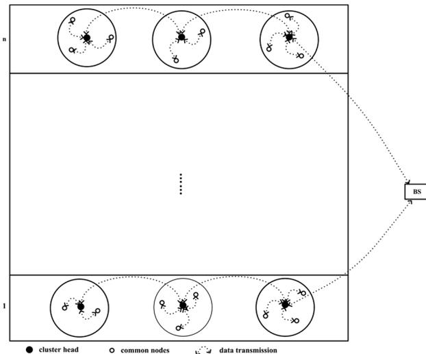
Fig. 4 The data transmission process of ICCHR algorithm
