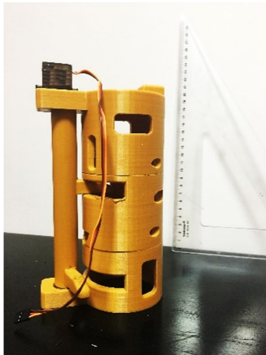
Fig. 11 Payload drop mechanism B fabricated via 3D printing
