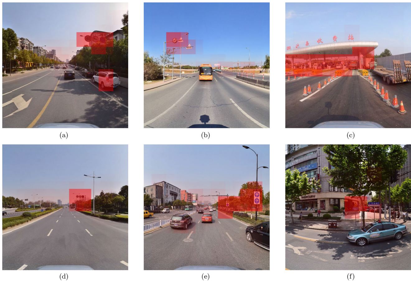
Fig. 4 Block score maps predicted by BlockNet. Blocks with deeper red coloring block with higher probability of containing traffic signs. These results demonstrate that our BlockNet produces correct block proposals. A great many irrelevant areas are filtered out; traffic signs occupy a relatively larger proportion of the block proposals.
