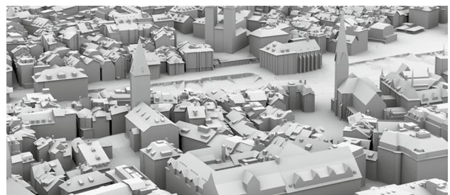
Fig. 2 3D city model with terrain, block and roof model (source: City of Zurich)
