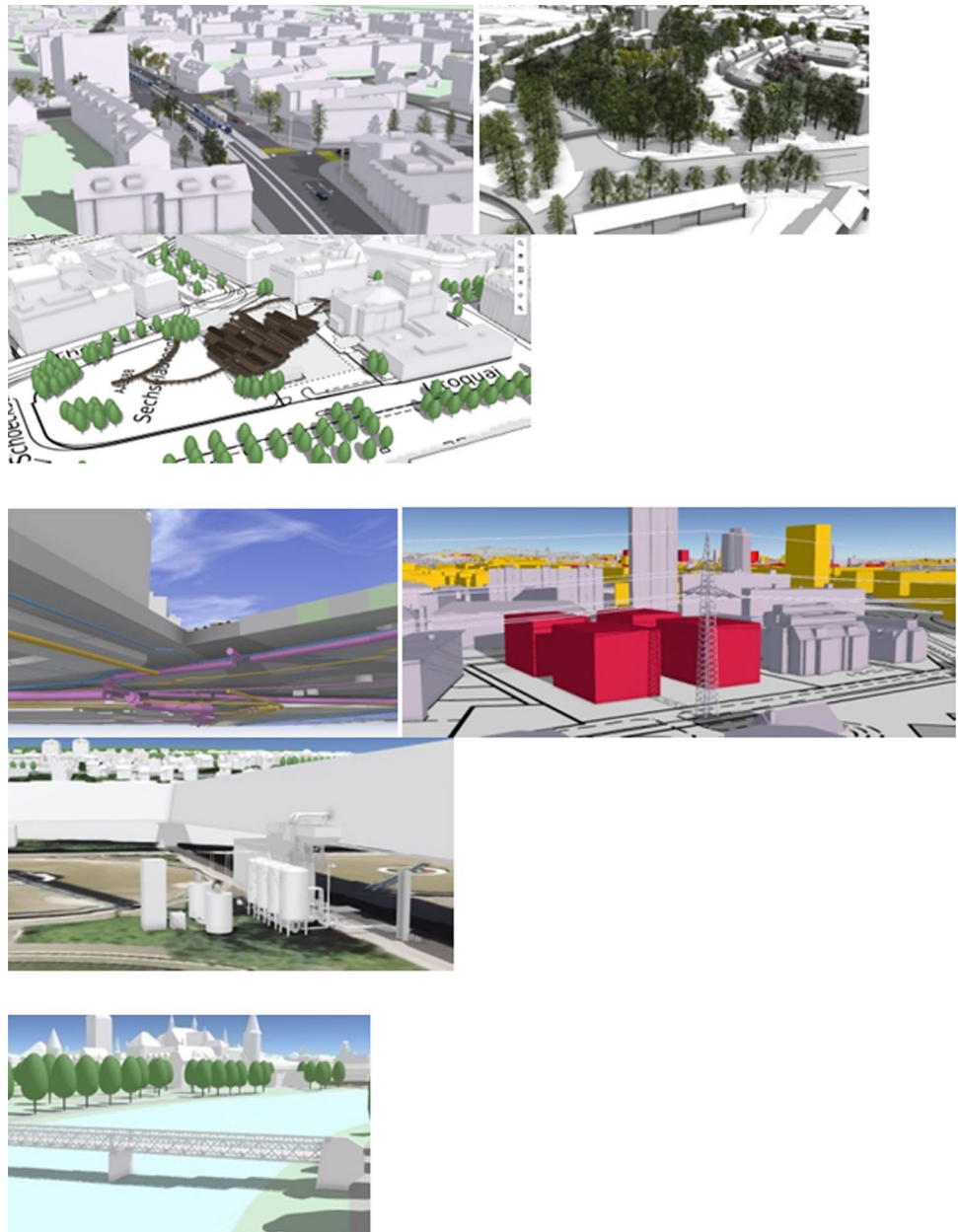
Fig. 3 Data levels and extensions of the digital twin: street space, trees, archaeological objects, underground, power lines, BIM model, bridges (source: City of Zurich)
