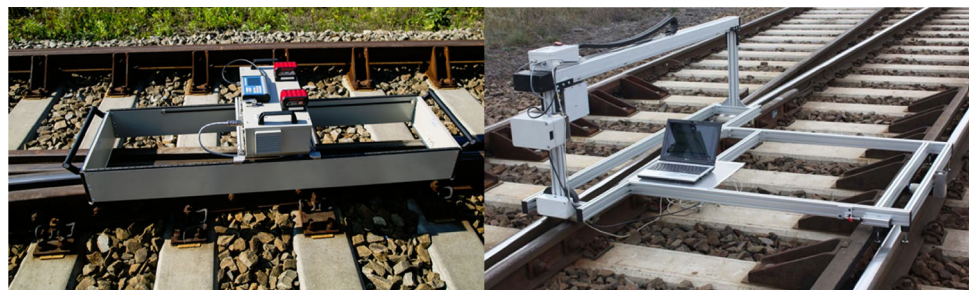
Fig. 2 Surface scanning methods for common crossings. (left, Scorpion [7]; right, Lauros [8])
