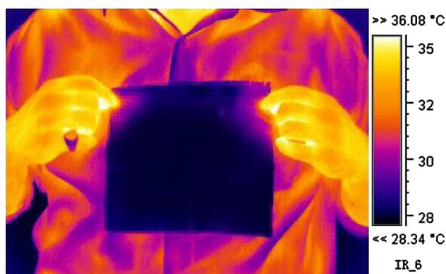
**Fig. 12** Captured thermal image from human body while keeping a piece of dense Cu–Ni–P–Ni composite nanoparticle-coated fabric
