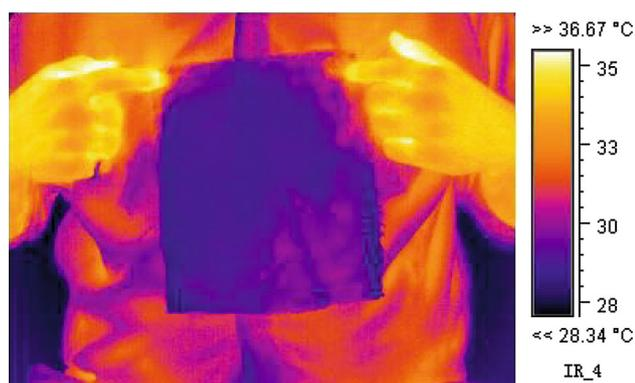
**Fig. 7** Captured thermal image from human body while keeping a piece of dense copper-coated fabric
