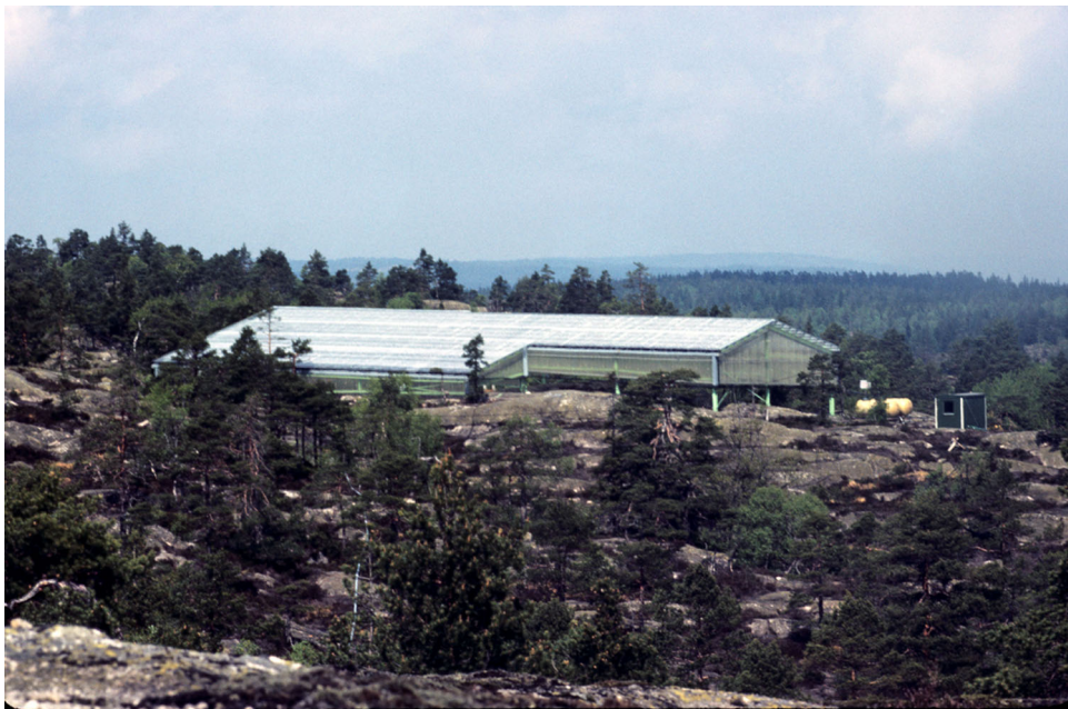
Fig. 7 Field experiments have played an important role for the overall understanding of the interactions between atmospheric deposition and ecosystem effects. The photo illustrates the covered catchment experiment to study the recovery of ecosystems at reduced emissions in Risdalsheia Norway (Photo NIVA)
