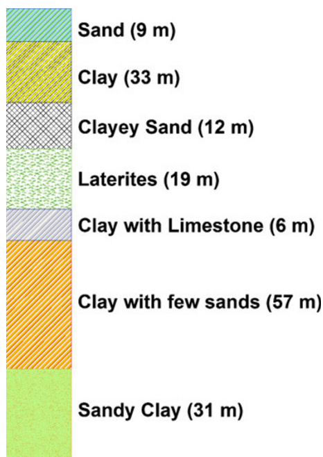
Fig. 2 Cross section of the under laying lithology
