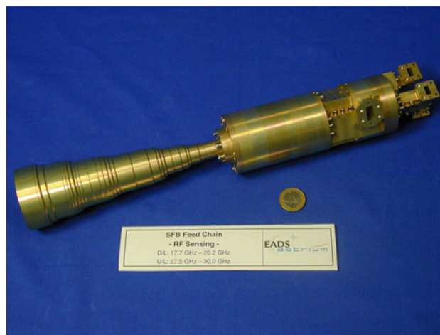
Fig. 5 Engineering model of an RF sensing feed chain
