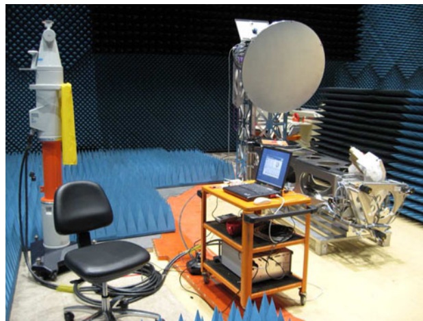
Fig. 19 Alignment of the Medusa feed system using laser tracker and positioner
