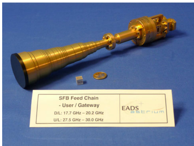
Fig. 3 Engineering model of a user gateway feed chain
