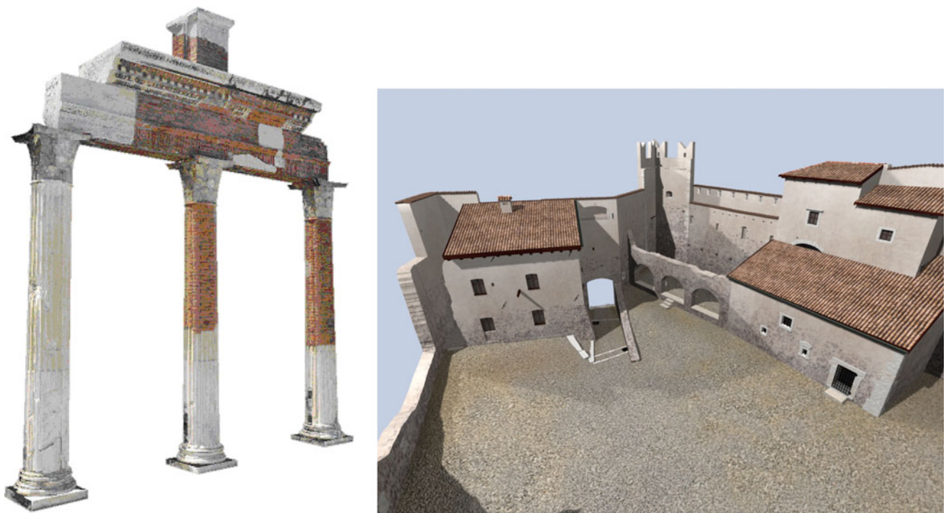
Fig. 5 Example of image-based 3D models of architectural structures derived using interactive measurements
