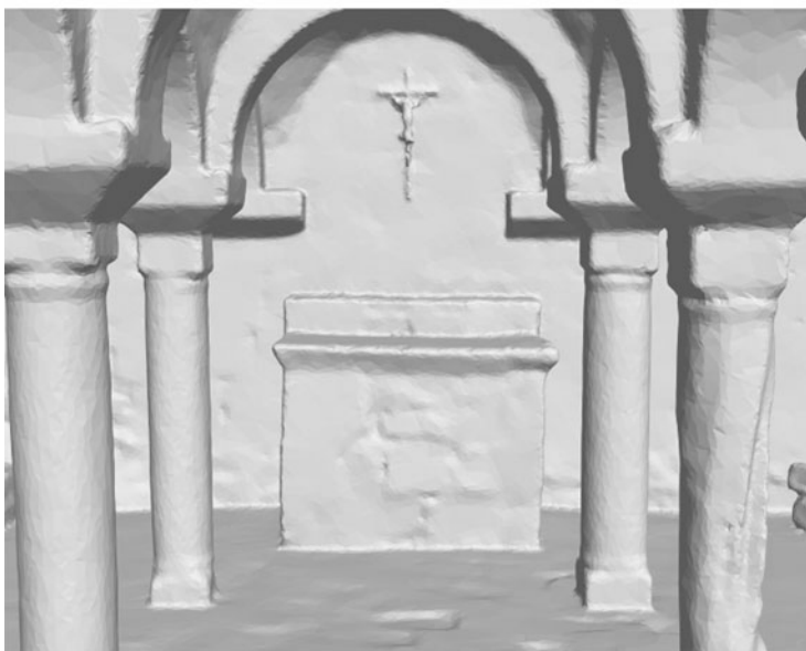
Fig. 2 Range-based 3D modeling of an underground church near Siena (Italy) and a Maya stela in Copan (Honduras)
