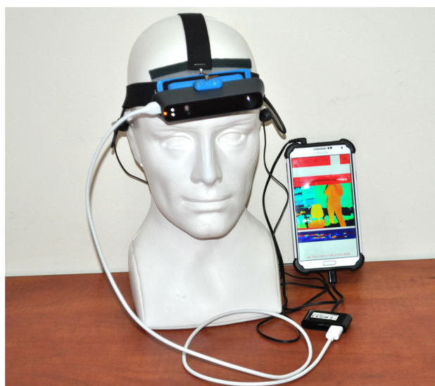
Fig. 2 Hardware components of the electronic system for interactive sonification of 3D scenes
