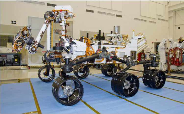
Fig. 4 Curiosity (flight) rover in Spacecraft Assembly Facility at the Jet Propulsion Laboratory with robotic arm deployed
