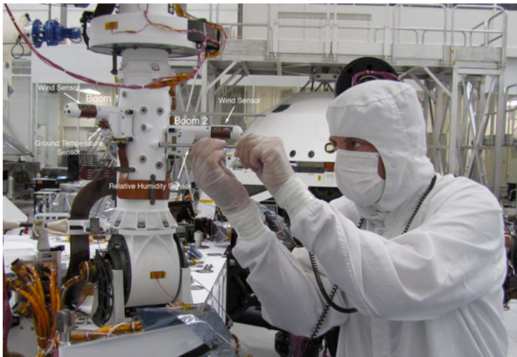
Fig. 28 REMS flight booms installed on a section of the rover mast. On the left is Boom 1 with wind and ground temperature sensor and on the right is Boom 2 with wind and humidity sensors. The humidity sensor itself extends downward from the boom and is hidden by the engineer's right hand . On both booms the conditioning electronics are located on the back, close to the attachment point on the mast
