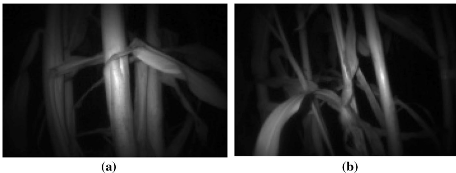
Fig. 10 Sample frames from the PMD depth sensor. The PMD was used to collect images at 15 fps and was mounted approximately 100 mm off the ground on the base of the robot to capture the second internode of the stalk
