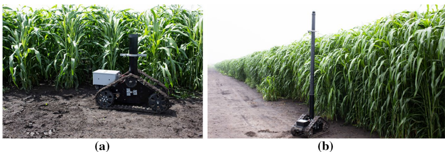
Fig. 1 Photos of the TERRA-MEPP phenotyping platform operating in the field: a with a short mast configuration used for imaging plants early in the growing season, and b with the first version of a fully extended mast for measuring the height of tall sorghum
