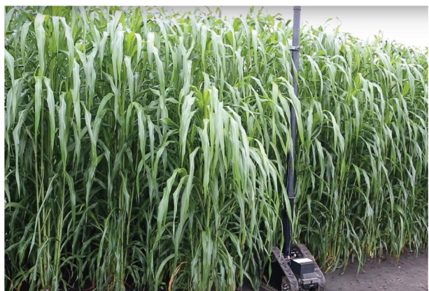
Fig. 9 The TERRA-MEPP platform being deployed in mature sorghum during August 2016. The top of the mast was raised above the canopy to its tallest height of 3.6 m above the body of the robot
