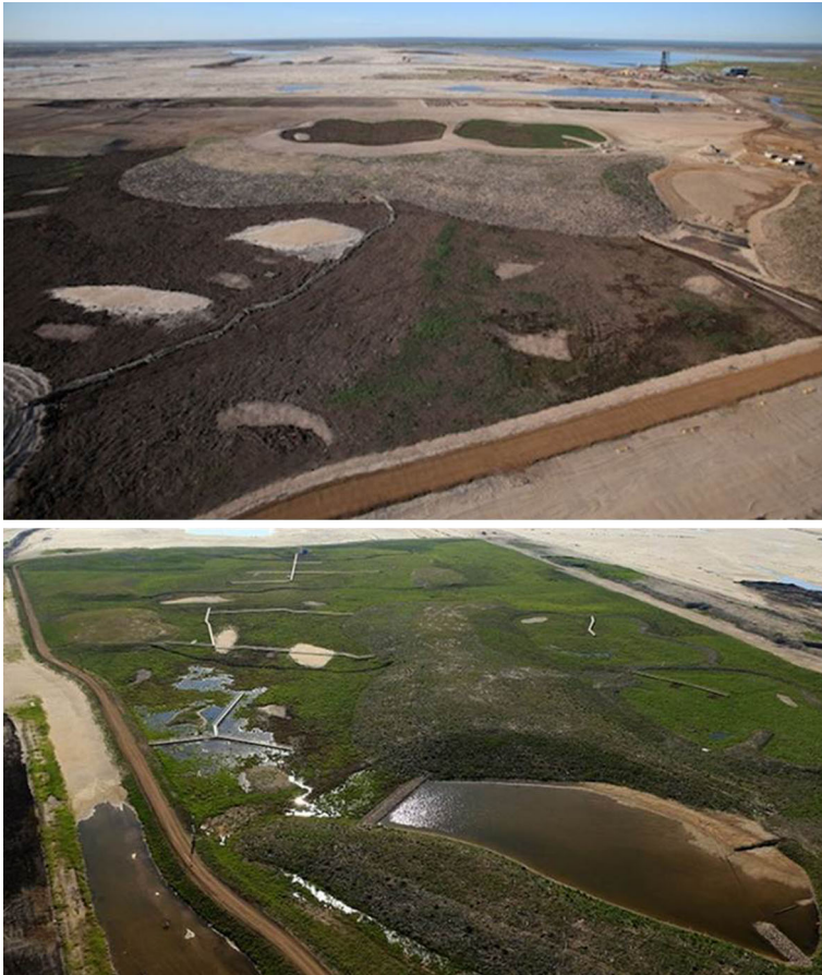
Fig. 1 Landform reconstruction, showing heterogeneity of materials and meso-topography, before ( above ) and after ( below ) revegetation after oil sands mining in Alberta, Canada. Photo courtesy of Syncrude Canada Ltd
