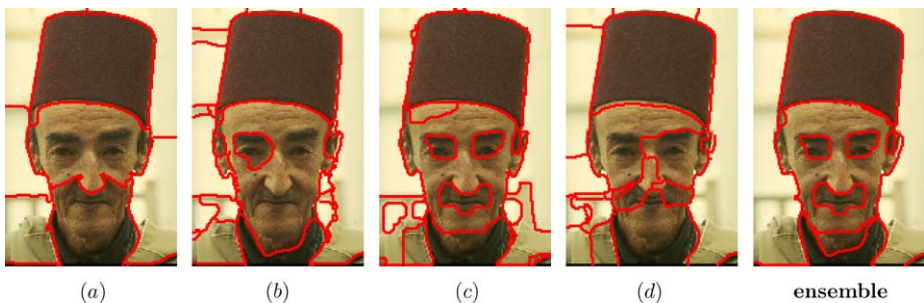
Fig. 7 A segmentation ensemble on an image from the Berkeley Segmentation dataset. (a)–(d) show the individual segmentations overlaid on the input image, the right-most image shows the segmentation generated from ensemble clustering. Segmentation methods used for (a)–(d) were (1), (3) with two parameter settings, and (4), see Sect. 8.2.2 for details
