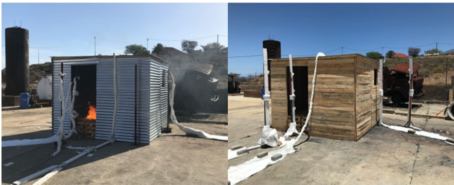
Figure 3. Steel clad dwelling setup (left image) and timber clad dwelling setup (right image).
