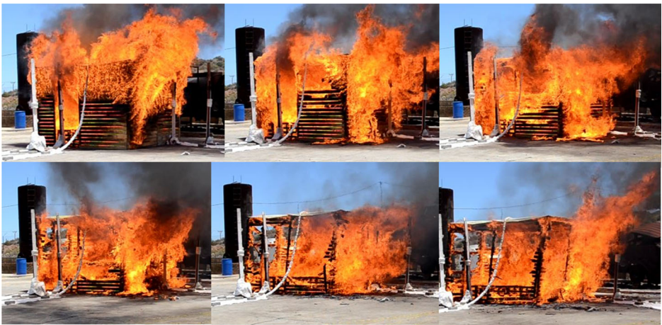
Figure 12. Ventilation openings forming in the timber clad dwelling experiment as a result of the cladding burning away, showing images at approximately 10 s intervals.
