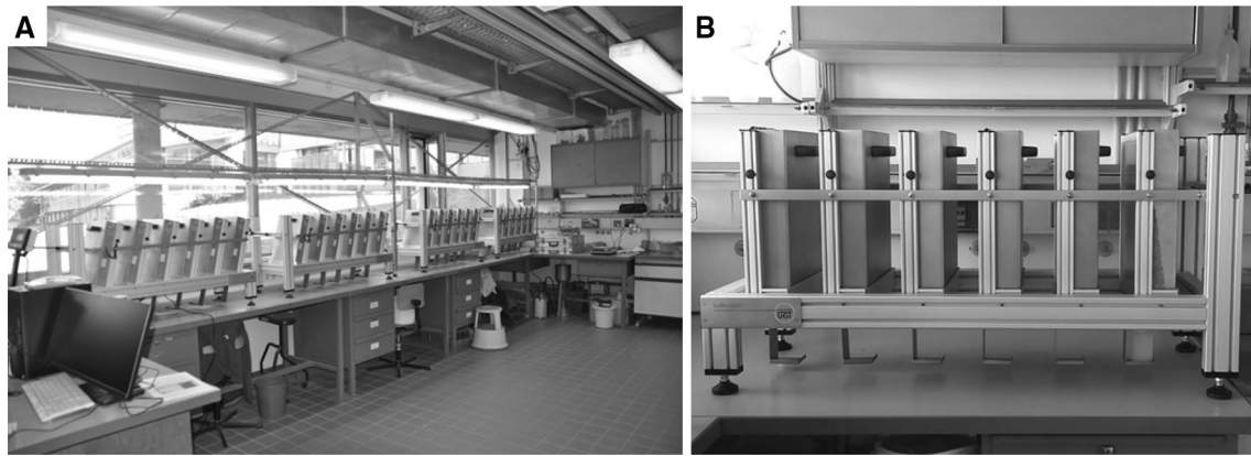
Fig. 1 a Soilinsight root growth-monitoring system comprised of 24 individual chambers placed on four separate frames. All chambers are inclined at 15°, b single frame holding six chambers placed in a vertical position at 0° inclination
