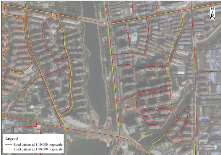
Fig. 1 The non-systematic discrepancies between road dataset at 1:10,000 map scale and road dataset at 1:50,000 map scale
