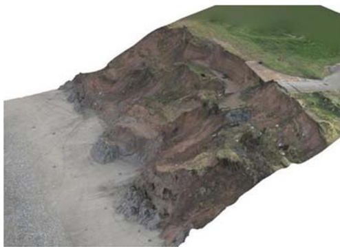
Fig. 13 Orthophoto image of coastal cliff landslide produced using UAV photogrammetry, Aldbrough, UK (2013), BGS©UKRI[2018]
