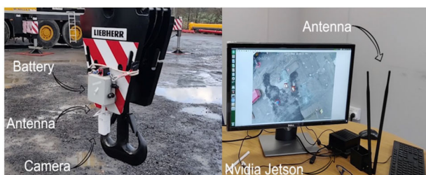
(a) Customised Camera mounted on the crane hook. (b) Deployed AI-based system.
