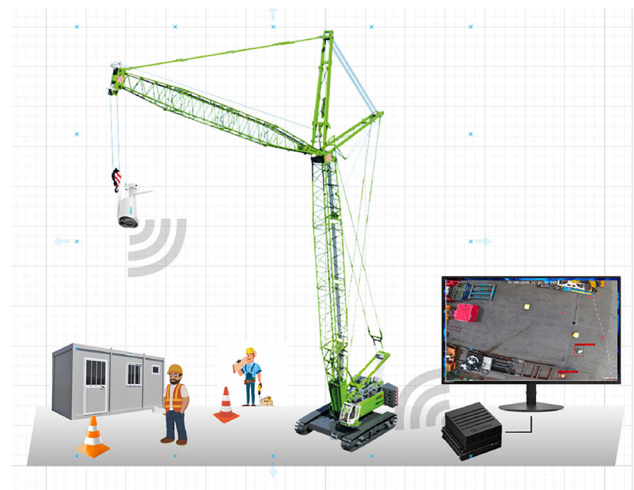
Fig. 2 The system for top-view detection of industrial sites. The system includes a video camera subsystem attached to the crane hook to capture and send the video stream to the small-form PC. The small-form PC hosts the machine learning platform and algorithms to detect the human objects
