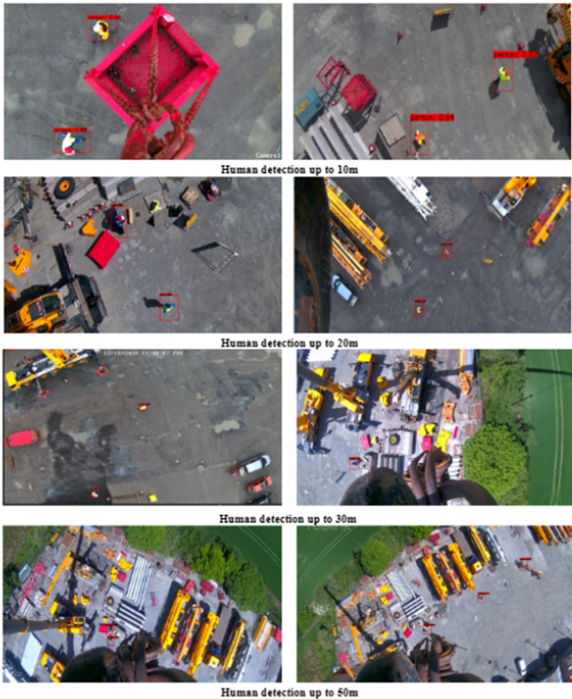
Fig. 7 Example of human detection at different altitudes in an industrial operational site. The images on the first row show the human detection up to 10 m; images on the second row show the
