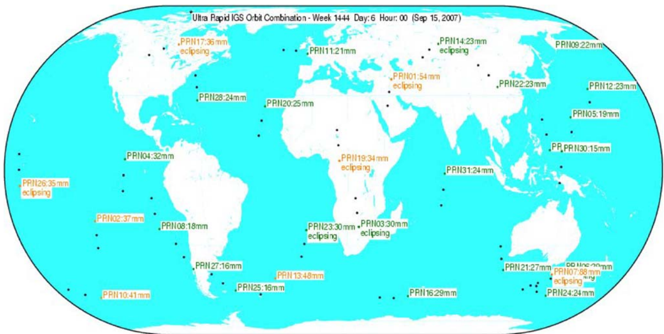
Fig. 3 Accuracy of a typical recent Ultra Rapid IGS orbit combination, by satellite
