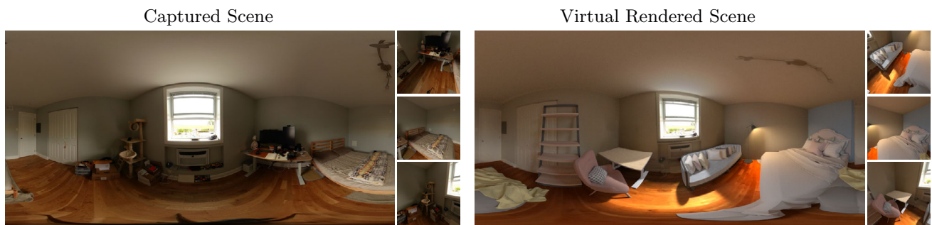
Fig. 1 Illustration of Our Rendering Approach: A real-world scene is captured at 11:27 AM (cloudy sky condition). Different furniture objects are removed from the existing room, and the empty scene is refurbished
