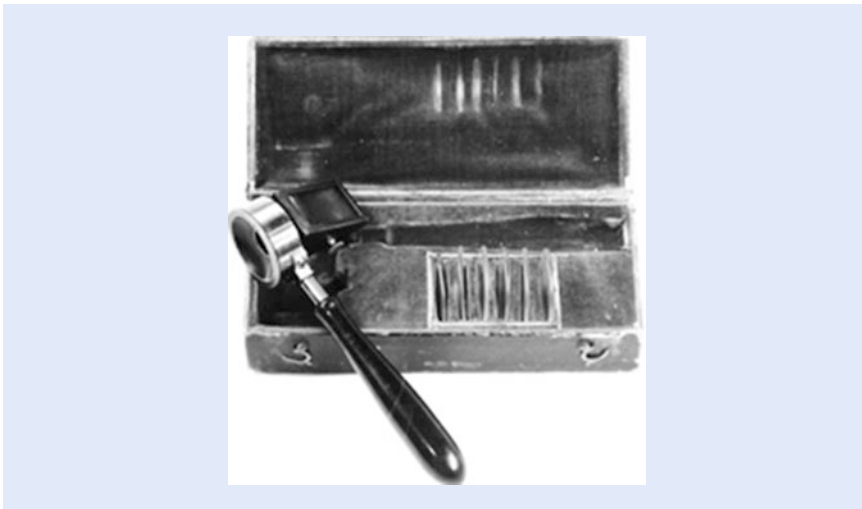
■ Fig. 13.4 Helmholtz ophthalmoscope (c. 1851)
