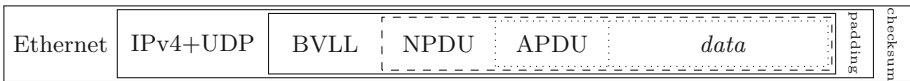
Fig. 3. Structure of a typical BACnet/IP packet. The outermost layer is the Ethernet layer, which encapsulates the Internet Protocol (IP) and User Datagram Protocol (UDP) layers. BACnet/IP is encapsulated within the UDP datagram as a BACnet Virtual Link Layer (BVLL), containing the BACnet Virtual Link Control (BVLC) that indicates the function of the BACnet packet. The presence of the Network layer Protocol Data Unit (NPDU) and the Application layer Protocol Data Unit (APDU) within NPDU depends on the particular BVLC function and the values in the Network Protocol Control Information (NPCI), which is the second octet of NPDU.
