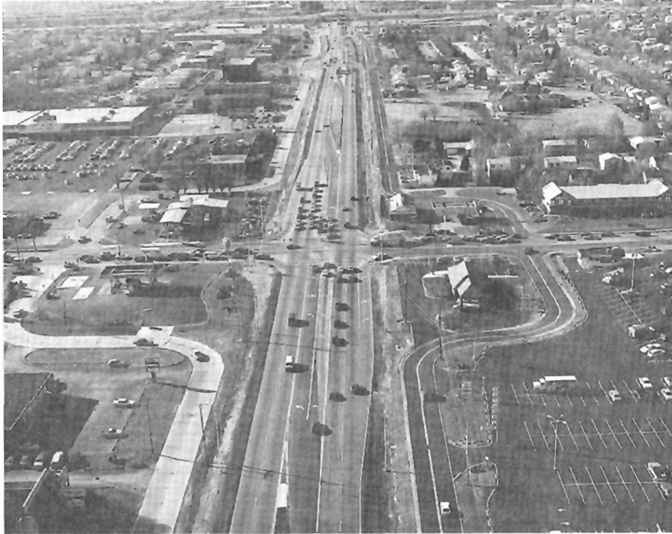
Exhibit 7-16. Divided Arterial Street With Two-Way Frontage Road
