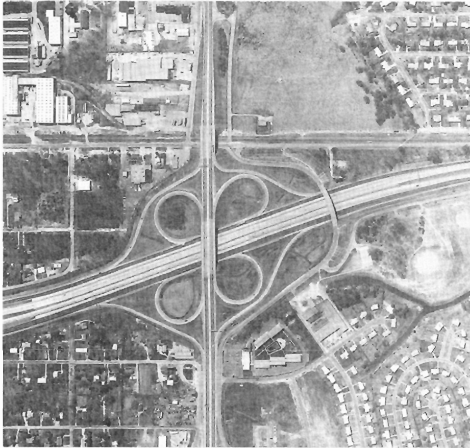
Exhibit 10-27. Cloverleaf Interchange With Collector-Distributor Roads
