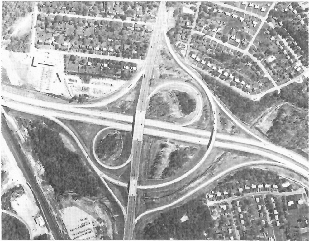
Exhibit 10-37. Semidirectional Interchange With Loops
