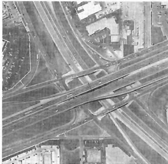
Exhibit 10-19. Freeway With a Three-Level Diamond Interchange
