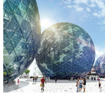
Nest by Robert Flottemesch, mono crystalline bifacial PERC solar modules, Annual capacity 6,633 MWh, LAGI 2019 Abu Dhabi
