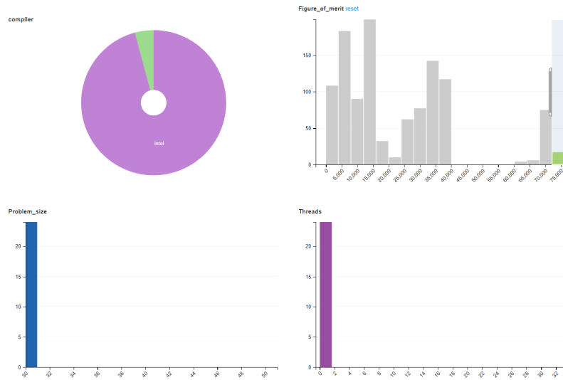
Fig. 2. The landing page charts from Figure 1 with a crossfilter applied. Selecting runs with highest FOM (top right) shows relationship to compiler (top left), problem size (bottom left), and threads (bottom right).
