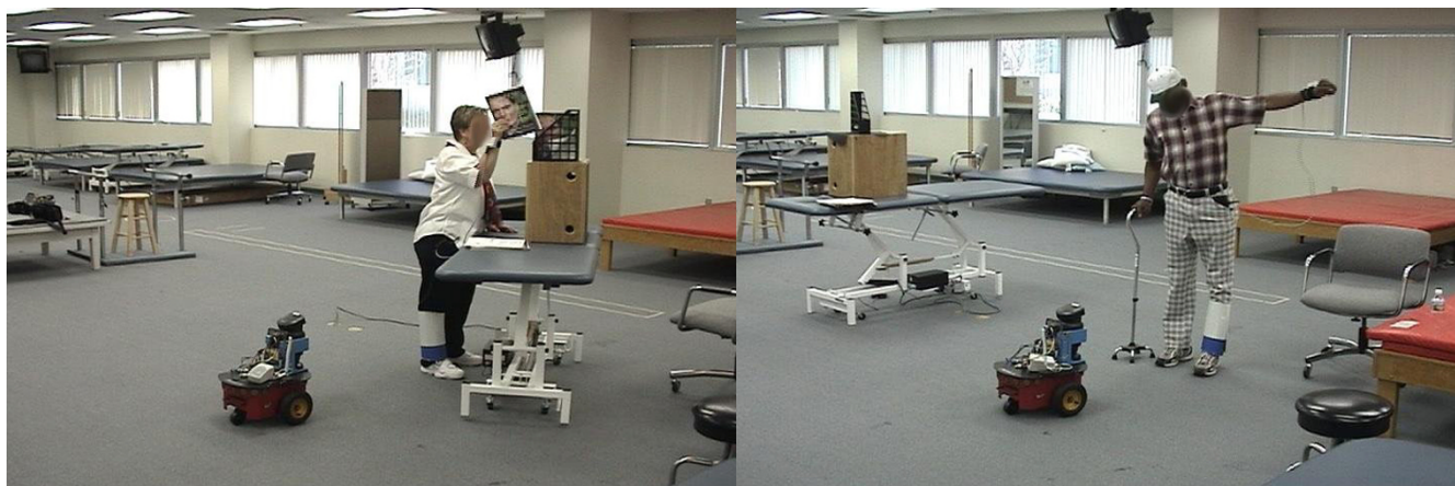
Figure 4 The two rehabilitation tasks: magazine stacking and free movement of the stroke-affected limb. The robot and participants during the two rehabilitation experiments: magazine stacking (left) and free movement exercises (right).
