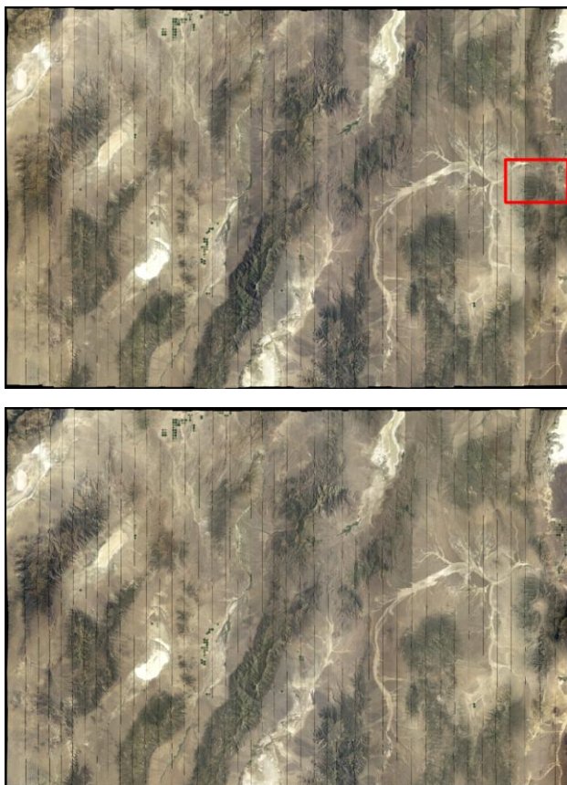
Figure 9. ADS100 ortho-image mosaic in Nevada. Top: image strips after atmospheric and BRDF correction; bottom: result of the radiometric normalization. The rectangle marks the area of Figure 10.
