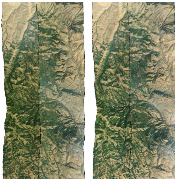
Figure 6. Comparison of radiometric normalization approaches for a section of an ADS ortho-image overlap of approx. 100,000 pixels along strip. Left: Result from the polynomial correction model of Gehrke (2010); right: result from the new radiometry fix approach with a spacing of 5,000 pixels.
