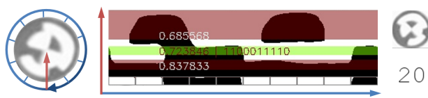
Figure 5: Histogram for an unrolled circular marker and rotation invariant binning of the code stripe. The numbers from top to bottom indicate the probabilities for center, binary code and outer circle. The marker with ID 20 has been successfully decoded.
