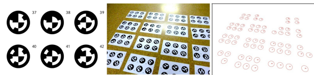
Figure 2: Fiducial markers, typical calibration image with printed marker sheets arranged on the planar surface of a floor and reliably detected markers with center position and ID.
