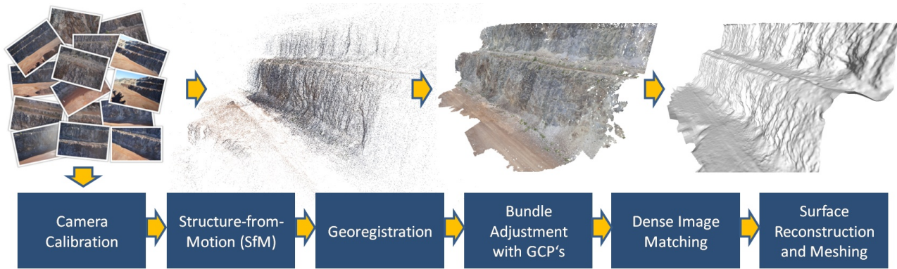
Figure 1: Automated processing workflow for precise and geo-accurate reconstructions. Top row: Image set, sparse reconstruction, dense point cloud and triangle-based surface mesh of a quarry wall in open pit mining.
