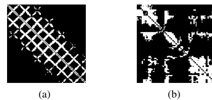
Figure 4: Rows and columns of the epipolar graph represent individual cameras and their connections to each other based on shared feature matches and image overlap. (a) shows a traditional aerial survey with regular flight pattern, (b) the connections between cameras for an unordered oblique image data set.
