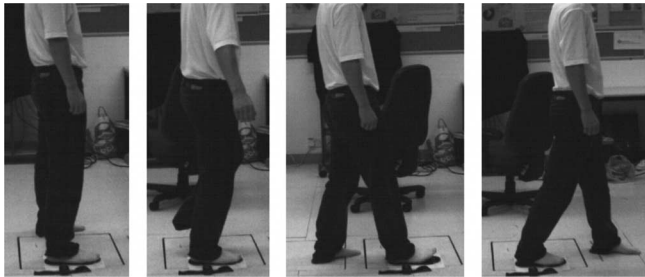
Fig. 11. Test actions: normal standing, standing on one leg, heel strike, and push off.
