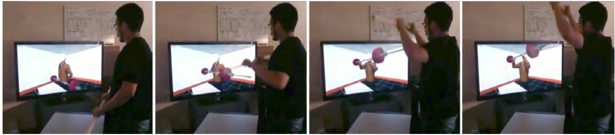
Figure 9: Virtual weightlifting task. The animation of the avatar is controlled by the user's actions and it is modulated according to the weight of the virtual dumbbell.
