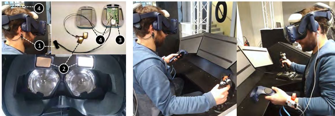
Figure 29: Experimental setup. Left, close-up of the Vive Pro Eye HMD with the additional hardware: (1) PPG sensor, (2), electrodes to assess the EDA, (3) electronic card, (4) 3D printed case. Right, overview of the VR setup in which the user is also equipped with the Shimmer3 GSR+ monitoring equipment.
