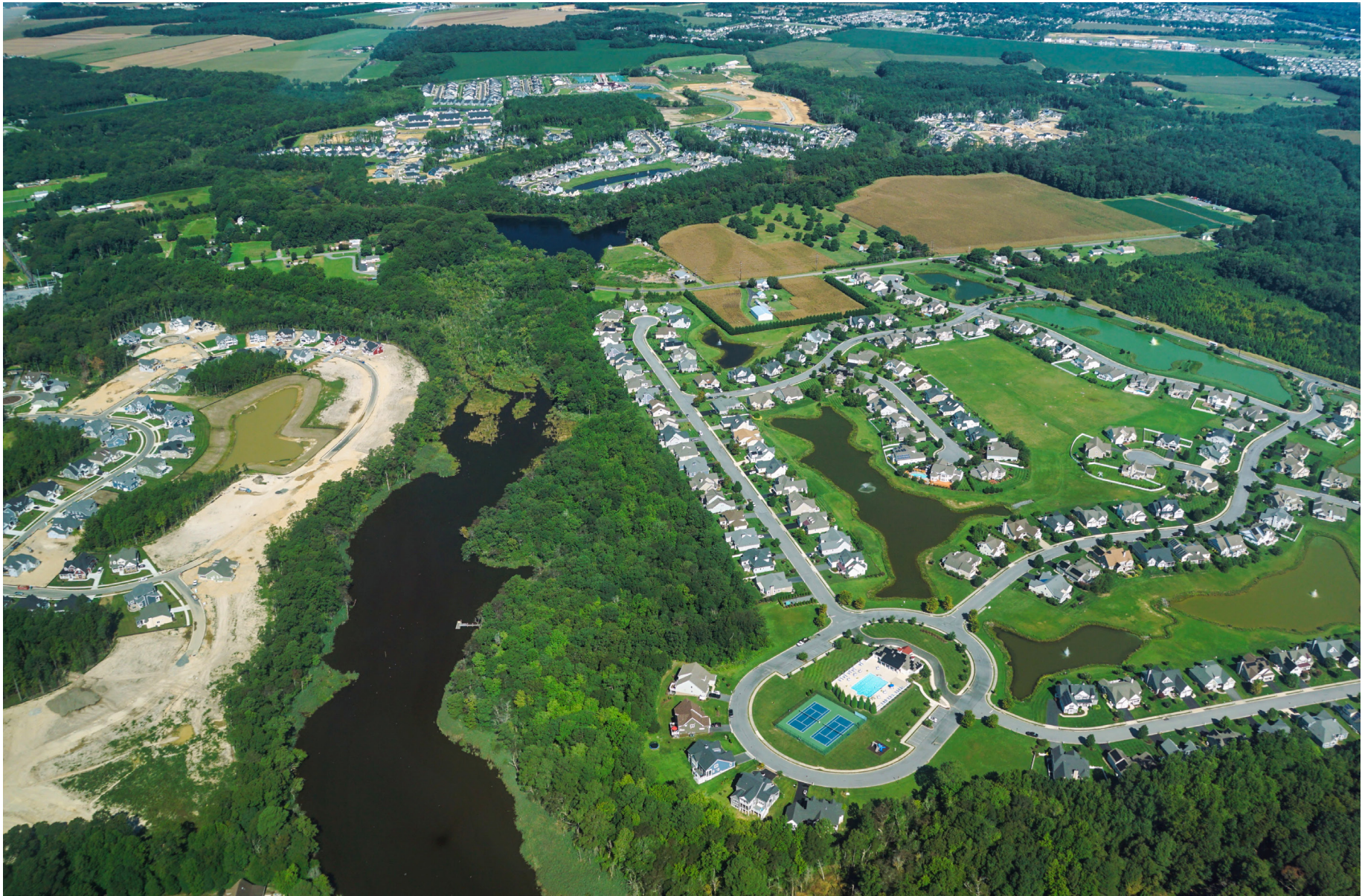
The wide forested buffer around the community at right provides much more protection to the waterway than the narrower one on the left.
