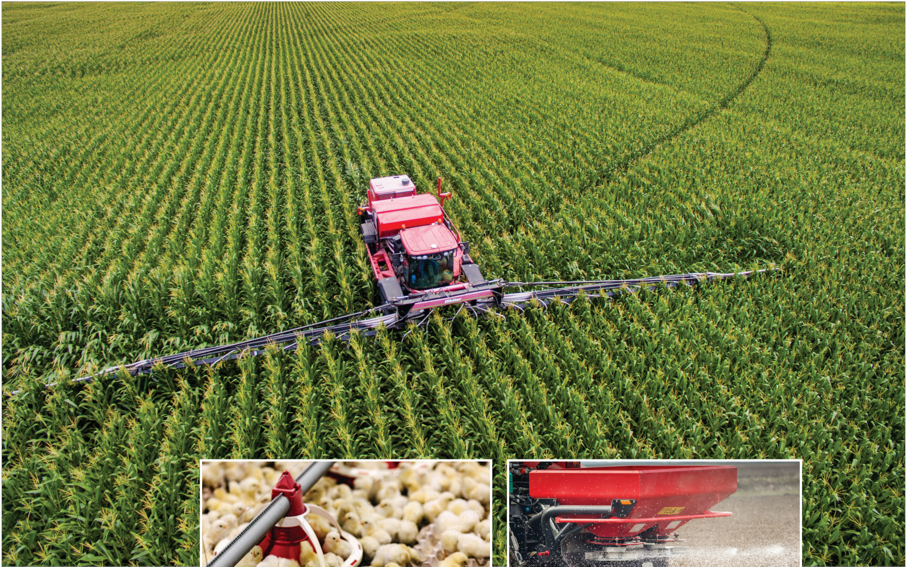
Air seeder sowing cover crop into corn. Photo courtesy Edwin Remsberg and USDA-SARE
