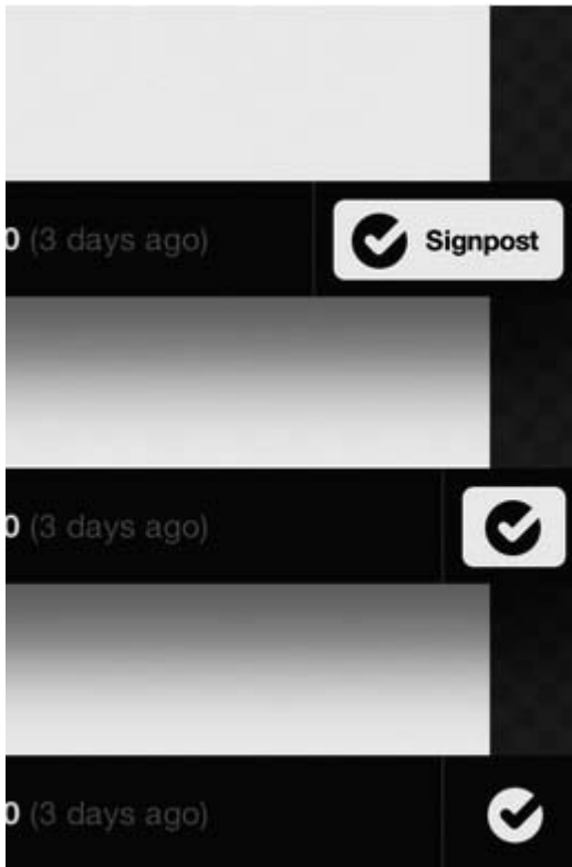
FIGURE 24.1 An example of progressive reduction—as the user learns the purpose of the button, he no longer needs to read the text, so the control changes.
