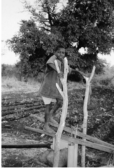
FIGURE 27.4 Operation of treadle pump.
