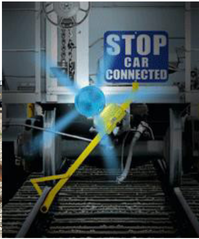
Night loading/unloading requires blue flashing light
