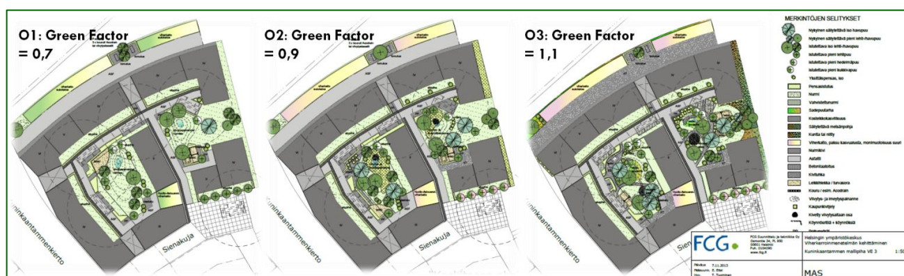
FIGURE 7: THREE LEVELS OF GREEN FACTOR CALCULATED FOR THE KUNINKAANTAMMI PILOT AREA O1: “AVERAGE”, O2: “MORE ECOLOGICAL THAN AVERAGE”, O3: “VERY ECOLOGICAL”.
