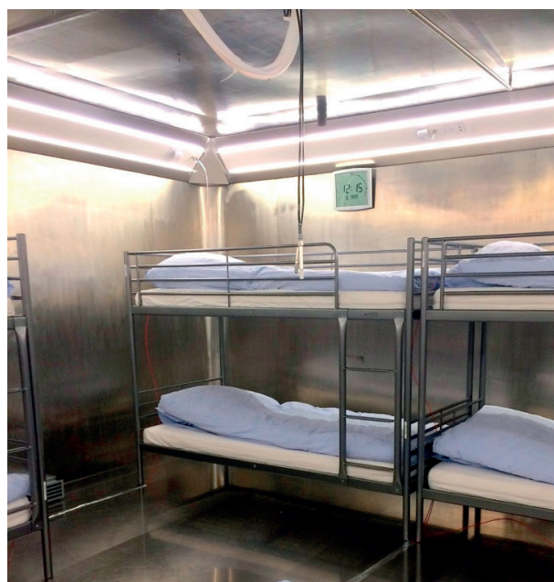
Figure 1. The exposure chamber equipped for overnighting used in the study on the effect of CO 2 during sleep on next-morning cognitive performance in schoolchildren (N = 36), Denmark
