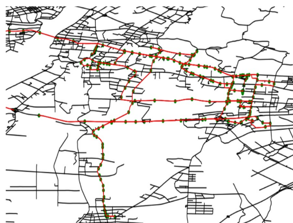
Fig. 2 Map matching results based on the trajectory points of representative trips. Black and red lines represent the road network and the trajectories after map matching, respectively. Green points represent raw taxi trajectory points
