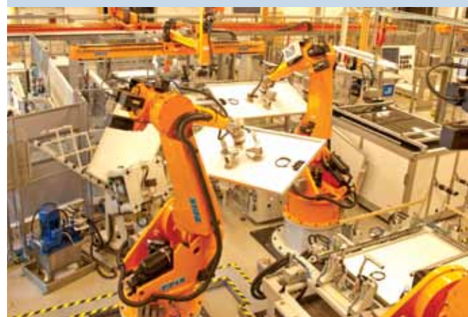
Fig. 5 - Fully automated final assembly of PV modules at the SweModule factory in Glava, Sweden (Photo: SweModule).
