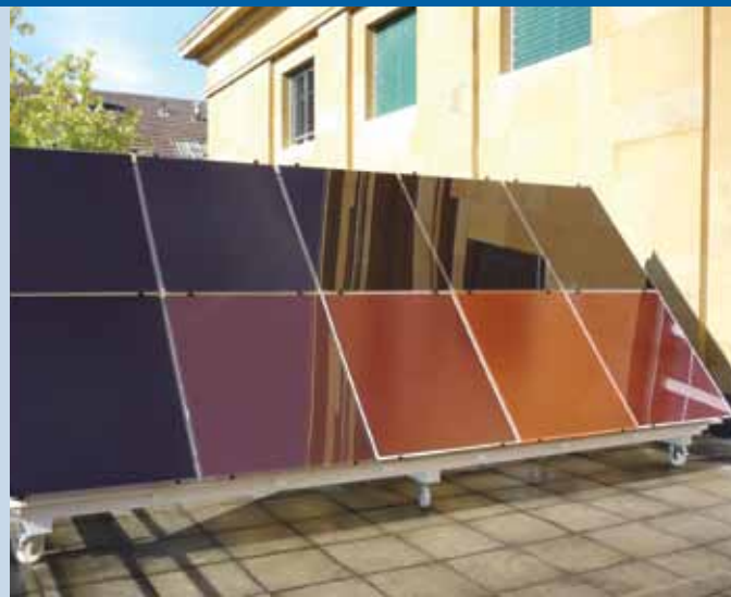
Fig. 3 - Coloured thin film BIPV modules are developed at the PV-Lab of EPFL (photo: EPFL).
